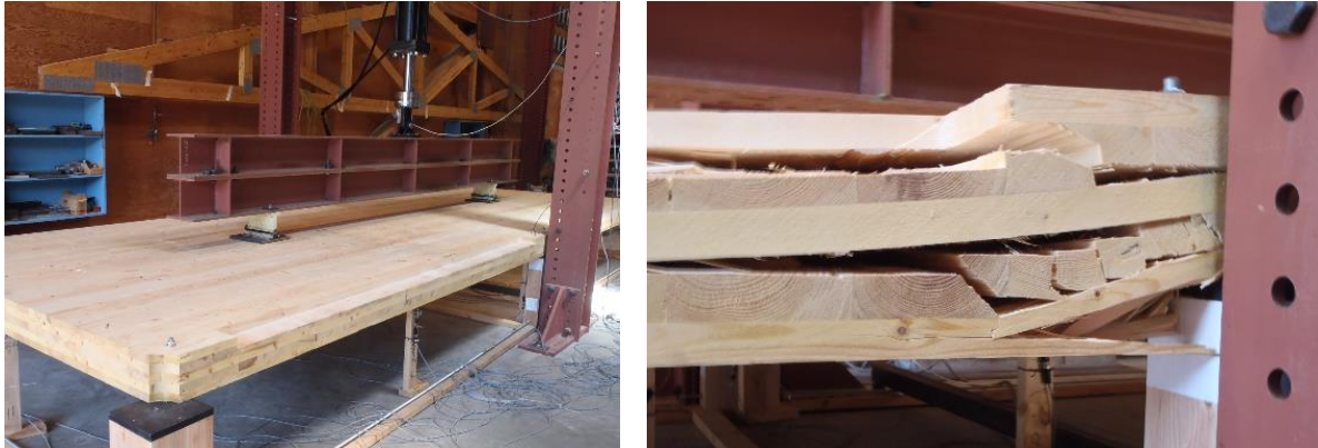
Figure 4: Point Supported CLT Panel Testing Apparatus and Failure.
